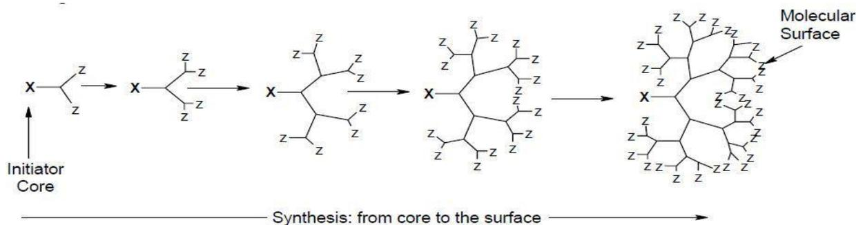
Figure 3: Divergent synthesis of dendrimer [15]
